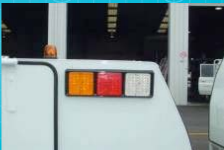
LED Assembly mounted to back panel
