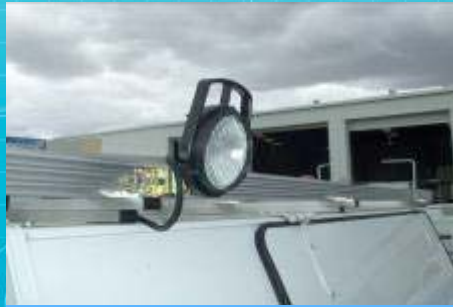
Swivel Work Lamp mounted to Ladder Rack
