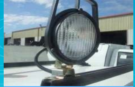
Swivel Work Lamp mounted to roof rack
