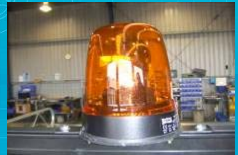
Amber Beacon mounted to roof rack
