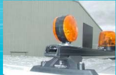
Front & Rear Facing Indicators mounted to roof rack
