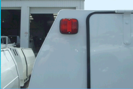
Brake/Tail mounted to back panel
