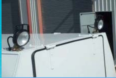
Swivel Work Lamp mounted to roof
