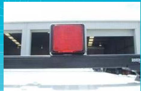
LED Brake/Tail Light mounted to roof rack
