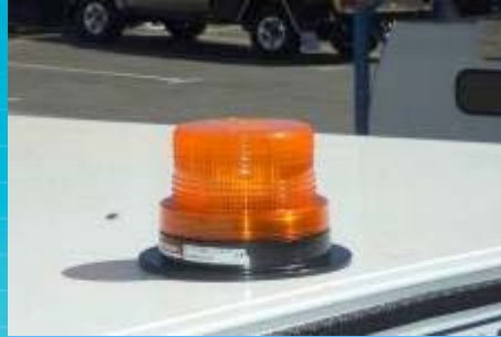
LED Amber Beacon mounted to roof
