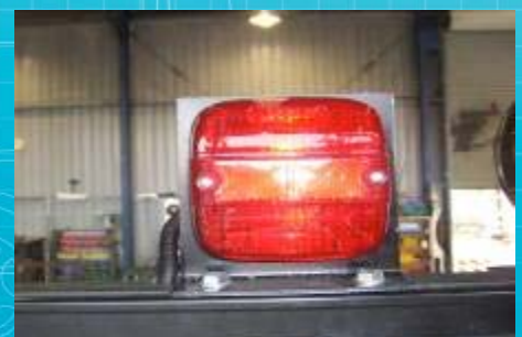
Brake/Tail Light mounted to roof rack
