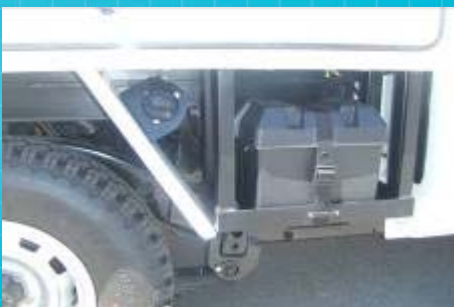
Underslung Battery Holder including Battery
