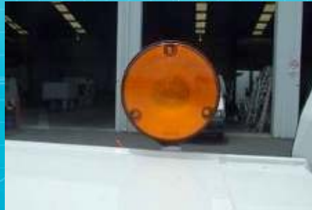
Front & Rear Facing Indicators mounted to roof
