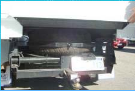
Spare Tyre mounted underneath
