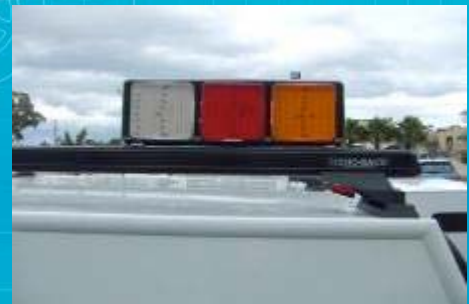
LED Assembly mounted to roof rack
