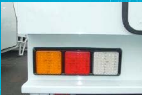
LED Assembly mounted to tail light press
