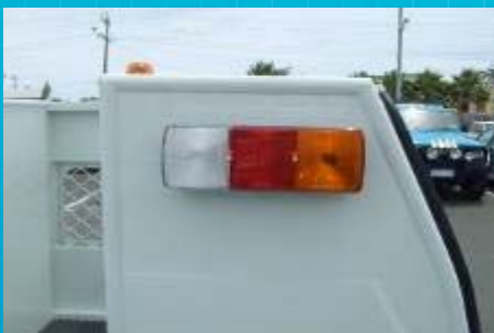
Assembly mounted to back panel
