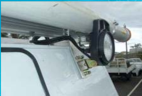
Swivel Work Lamp mounted to side panel
