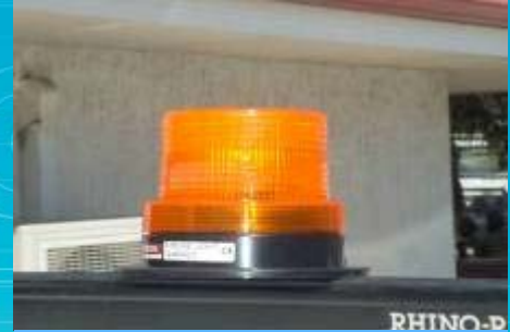
LED Amber Beacon mounted to roof rack
