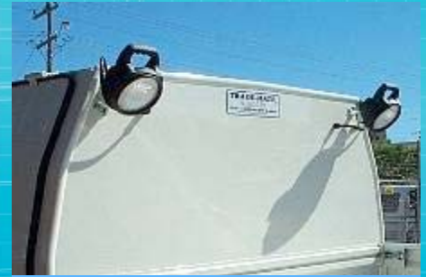
Swivel Work Lamp mounted to back panel
