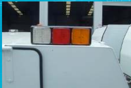
LED Assembly mounted to roof
