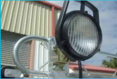
Swivel Work Lamp mounted to Tradesman Rack
