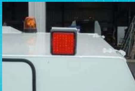
LED Brake/Tail Light mounted to roof
