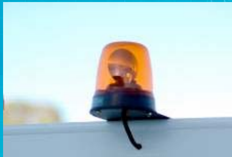
Amber Beacon mounted to roof
