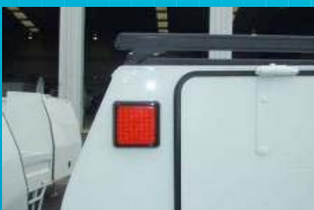
LED Brake/Tail light mounted to back panel
